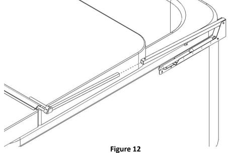
13. Prior to this step, ensure that the cover is centered on the spa (in closed position). Securely fasten the Stabilizer Bars (cvFF) **and** the Extension Arms (cvDD) to the Pivot Arms (cvCC) with the Medium Hex bolt (cvD). Tighten the bolt to the pre-installed nut on the Pivot Arm (cvCC) so that the Extension Arm (cvDD) will no longer slide in the Pivot Arm (cvCC) and the Stabilizer Bar (cvFF) does not move freely. **Do Not Over Tighten the Bolts.** See Fig 13.
