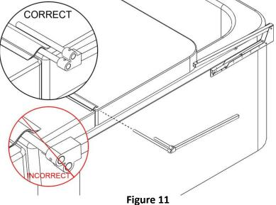
12. Align the Extension Arm (cvDD) so that it will slide into the Pivot Arm (cvCC). Slowly and evenly slide the Pivot Arm (cvCC) into the Extension Arm (cvDD) until the spa cover is centered over the spa, as shown in Fig 12.
