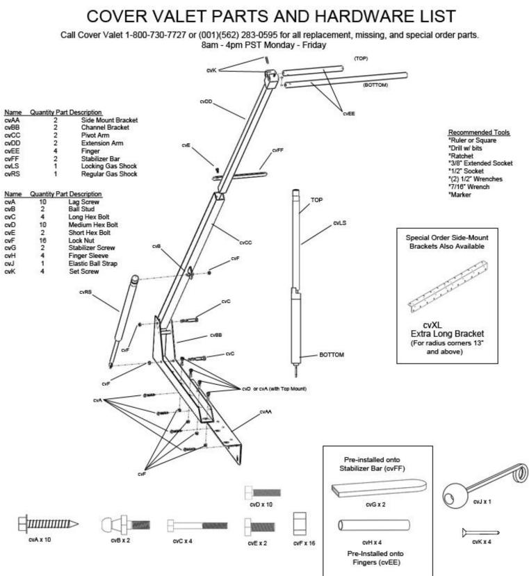
2. Attach the Ball Stud (cvB) to the Pivot Arm (cvCC) with the Lock Nut (cvF); repeat this for each side of the spa. Ensure the round part of the Ball Stud (cvB) is facing away from the spa. See Fig 2.
