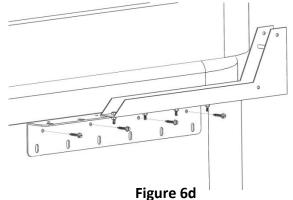
You may have some parts left over: 2 Lag Screws (cvA) and possibly 2 Medium Hex Bolts (cvD) with 2 Lock Nuts (cvF), depending on the offset of the Channel Bracket (cvBB) and the Side Mount Brackets (cvAA).
