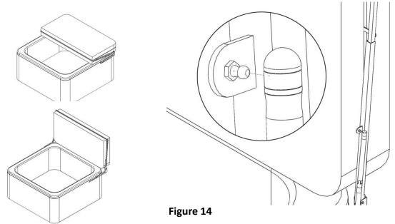
Repeat this step on the other side of the spa with the Locking Gas Shock (cvLS).
