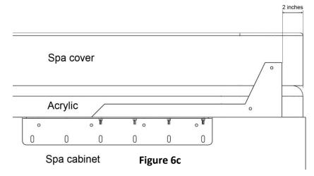
d. Use the 4 Lag Screws (cvA) to mount the Side Mount Bracket (cvAA) to the side of the spa. Repeat Steps 6a through 6d on the other side of the spa. See Fig 6d. After you install the Lag Screws (cvA) tighten the Medium Hex Bolts (cvD) and Lock Nuts (cvF) holding the brackets together.
