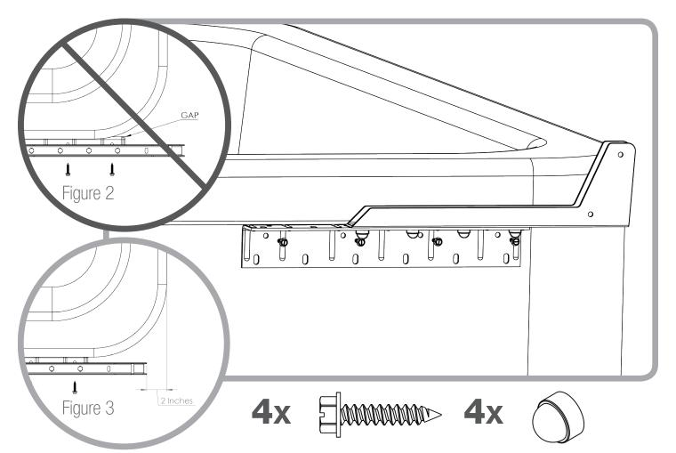
Place the assembled bracket against the side of the spa. The Side Mount Bracket (prAA) must be flush with the side of the spa. <u>DO NOT allow the Side</u> Mount Bracket (prAA) to hang over the rounded edge.(See Figures 2 and 3)
