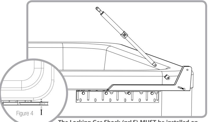
The Locking Gas Shock (prLS) MUST be installed on the side of the spa where you will operate the lift.
