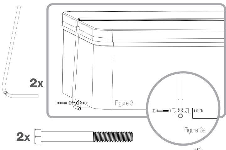
Connect the Pivot Arm (crDD) by placing one Plastic Pivot (crGG) on each side of the hole in the Pivot arm (crDD) then attach it to the Base Plate using a 3/8" x 3-1/2" Hex Bolt (crC), (2)Flat Washer (crB), and 3/8" Nylon Locknut (crC) as shown in Figure 3 & 3a.
