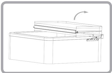
Fold Back the spa cover then manually lift the Cover Valet and spa cover to the upright position.
